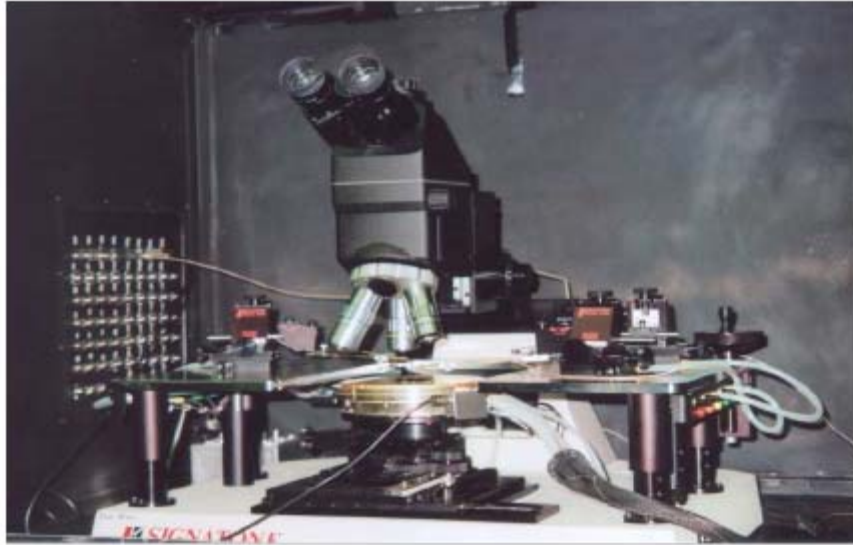
Figure 5. Black box and equipment inside used for testing [5].
