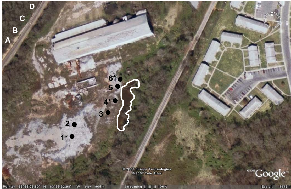
Figure 4.1. Satellite image of the abandoned Smokey Mountain Smelter site in South Knoxville, TN, USA (Image from Google™ Earth). The large building on the property houses two rotary furnaces and an incinerator. Slag from the smelting process now exists in piles over much of the property. Numbers 1-6 and respective black spots designate plots of Pteris cretica plantings and slag sampling. The white line outlines the waste lagoon. Letters A-D indicate approximate locations of uncontaminated soil sampling. The right side of the image shows the adjacent public housing project.
