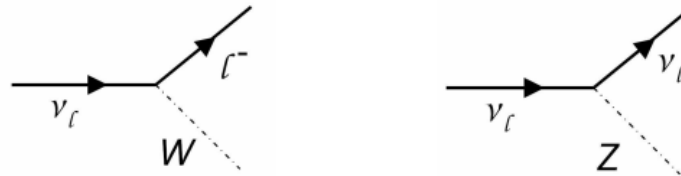
Figure 2.2 Weak interactions of the neutrino. Charged current interaction (left) and neutral current interaction (right).
