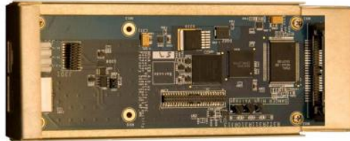
Figure 4.11. NOvA's front end board, the component that processes signals from the APD pixels and extracts time and amplitude data which it transmits to the data concentrator modules.
