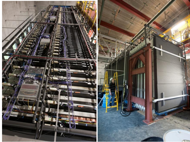
Figure 4.12. The NDOS. Left: The top of the detector. The DCMs are visible, as well as the FEB and APD electronics boxes. Right: The full detector. [63]
