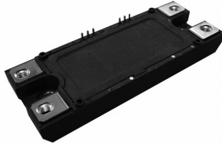
Figure 2-6. 1200 V / 120 A SiC MOSFET module [41].
