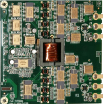
Figure 2-10. Commercial high temperature SOI gate driver [55].
