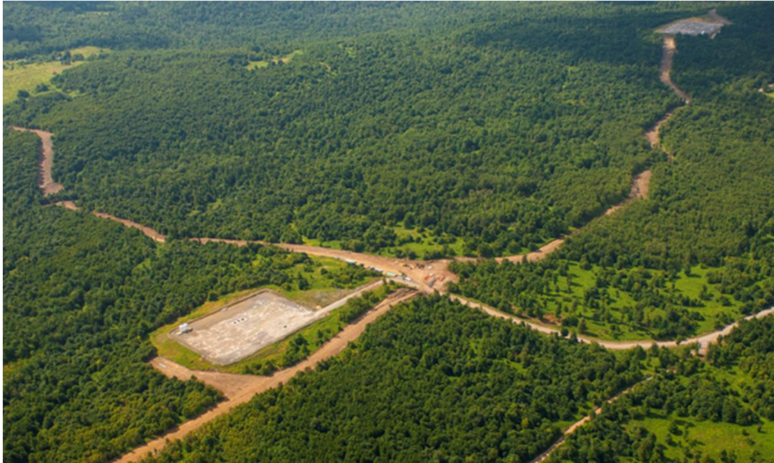
Fig. 2.1. Well pads (rectangular clearings), access roads (linear clearings in bottom-right), and gathering pipelines (other linear clearings) pose many impacts on habitats in the Marcellus formation, including forest and wetland loss and fragmentation, displacement of species of conservation concern, erosion, and freshwater sedimentation and fragmentation. Courtesy of M. Godfrey, The Nature Conservancy.
