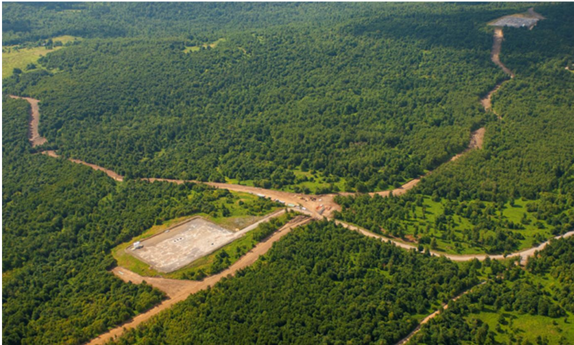
Fig. 3.1. Well pads (rectangular clearings), access roads (linear clearings in bottom-right), and gathering pipelines (other linear clearings) pose many impacts on habitats in the Marcellus formation, including forest and wetland loss and fragmentation, displacement of species of conservation concern, erosion, and freshwater sedimentation and fragmentation. Courtesy of M. Godfrey, The Nature Conservancy.
