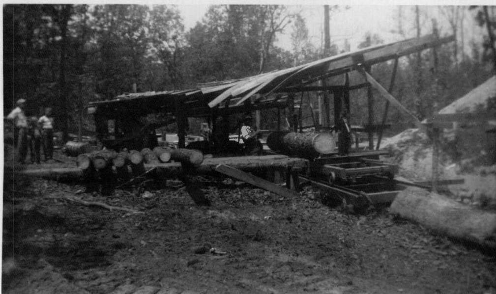
Figure 50. A small portable mill sawing pine logs in the Catoosa Wildlife Management Area.
