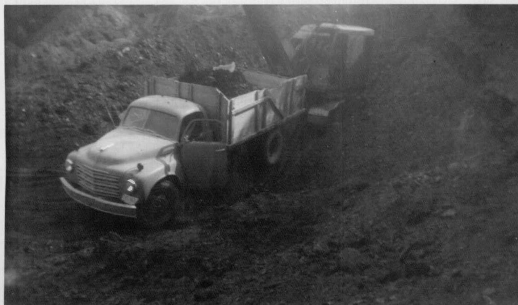
Figure 57. Loading coal in a strip mine in the western edge of the Crab Orchard Mountains area.
