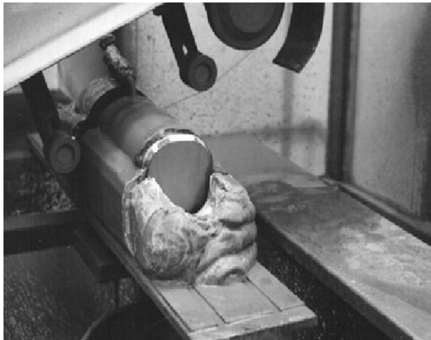
Figure 2.7: Germanium crystal being sliced [21].
