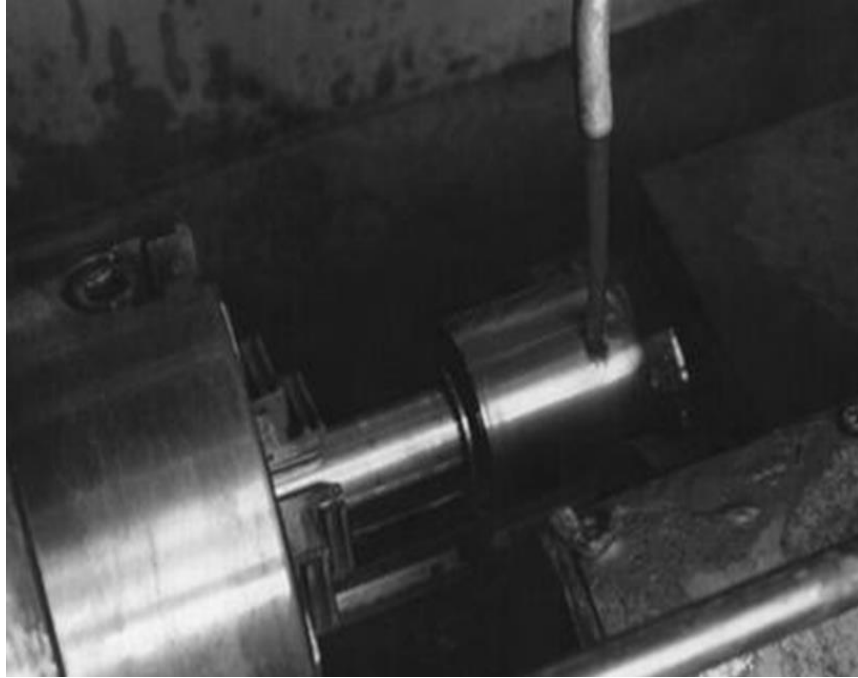
Figure 2.8: Germanium crystal being ground [21].
