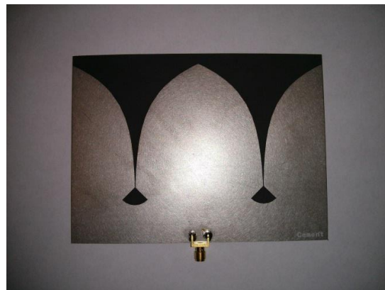
(d) Antenna designed with cement wall
