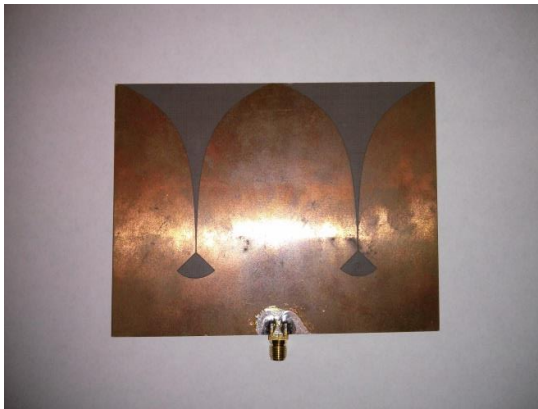
(a) Antenna designed in free space
