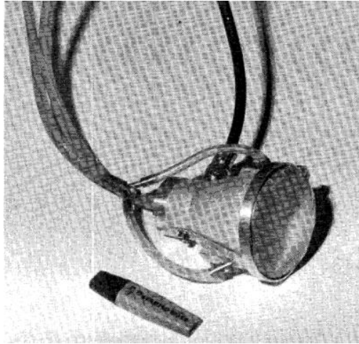
Figure 2.5 The water-filled applicator reduces reflection and provides variable surface cooling on the interface.
