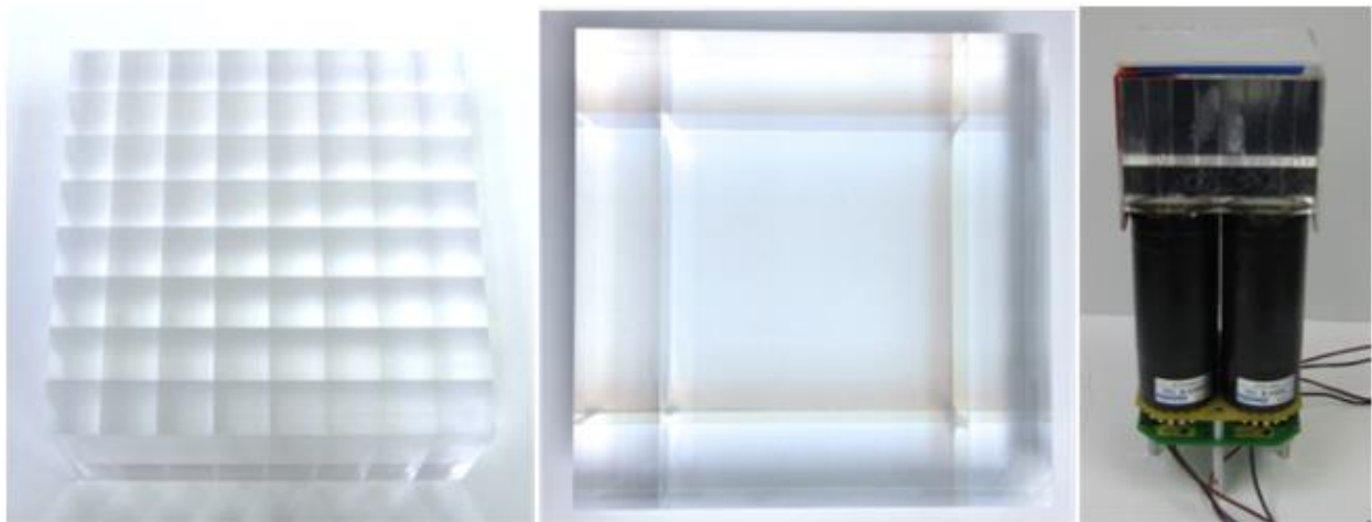
Figure 26. EJ-299-34 segmented pixel array (left), segmented light guide (middle), assembled detector module (right).
