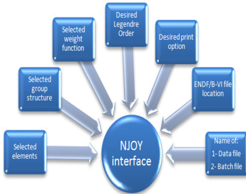
Figure A-5 "NJOY99" interface that generate elemental group microscopic cross section
