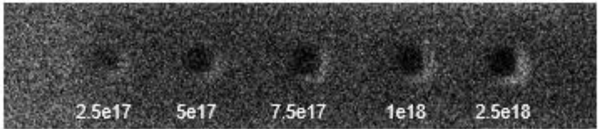
Figure 3.34. NIM image for a dose study of neon in a copper structure (Cu/SiO 2 /Si).
