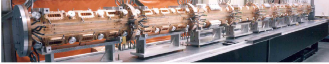
Figure 17. The LEDA coupled RFQ - After [16].
