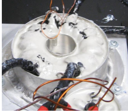
Figure 1.19. DC CM choke with cooling design
