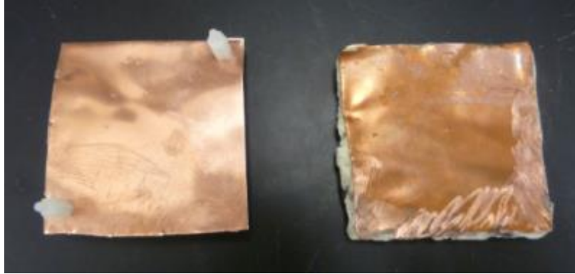
Figure 6.7. Example capacitor built by potting material vs. air capacitor
