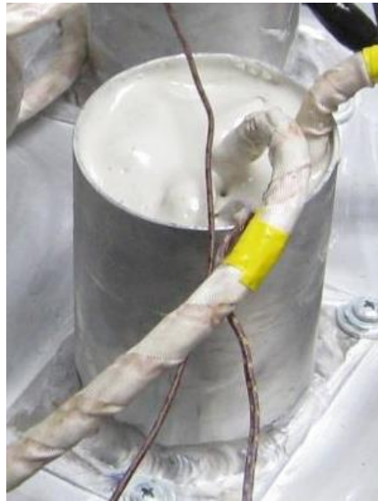
Figure 6.6. DM inductor in cooling case with potting
