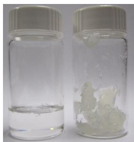
Figure 4. 3: Picture of MPBd-OH-2 (liquid) and MPBd-UPy-2 (non-flowing semisolid)
