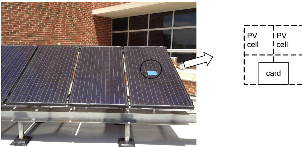
Figure 4.33. PV panels of phase a : two cells of the third panel are partly covered.
