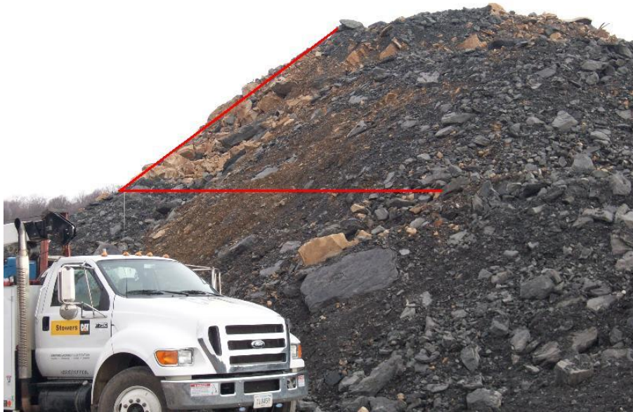
Fig. 2.5. Typical field determination of the angle of repose at National Site (White et al. 2009). Camera placed on a level and photo taken of material in loose state. Note the large number of oversize ( > 0.3 m) particles in the reclaimed material.
