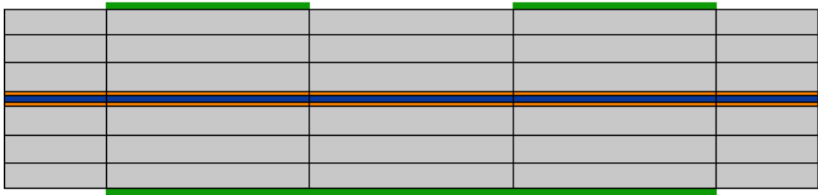
Figure 4-2: Computational domain that represents the asymmetric case. Green boundaries represent prescribed temperature boundary conditions. Grey areas represent the DM, orange areas represent the catalyst layers, and the blue area the membrane.
