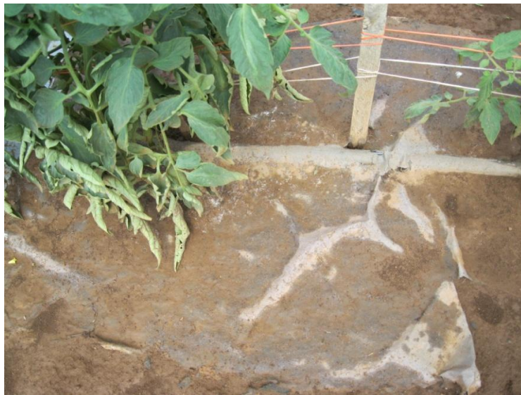
Figure 1: WeedGuardPlus®, a cellulosic mulch, in the open field showing premature degradation
