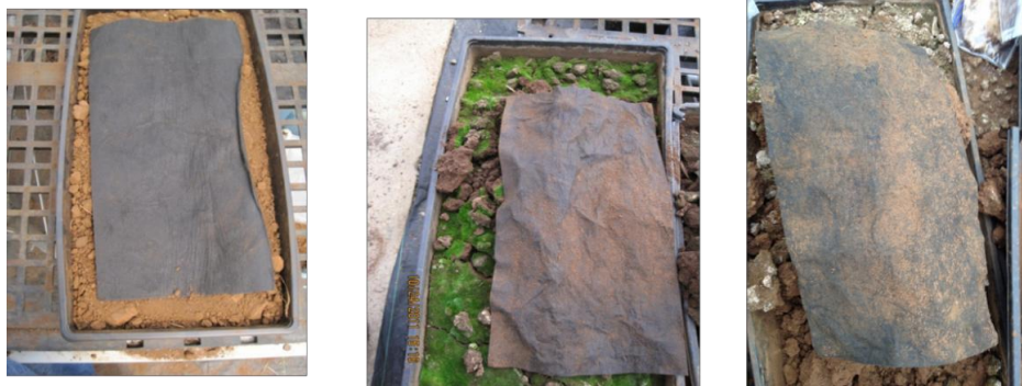
Figure 18: Visual observation of SB-PLA-2011(black) retrieved from burial in soil (Study 2) treated with LWDR + PJ at 0, 10, and 30 wk (left to right)
