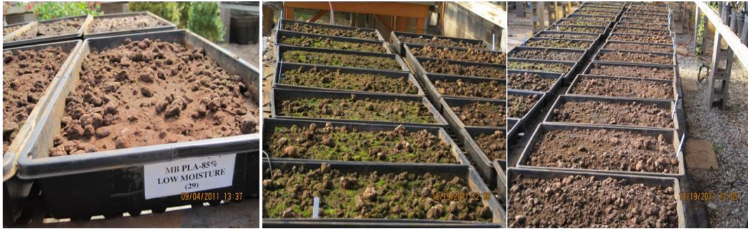
Figure 13: Plastic trays containing mulches buried in soil and compost mixture arranged in randomized block experimental design with the experiments conducted in a greenhouse (Study 2)
