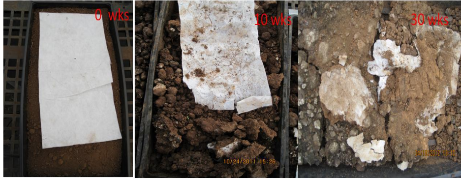
Figure 16: Visual observation of MB-PLA retrieved from burial in soil (Study 2) treated with LWDR+PJ at 0, 10, and 30 wk (left to right).
