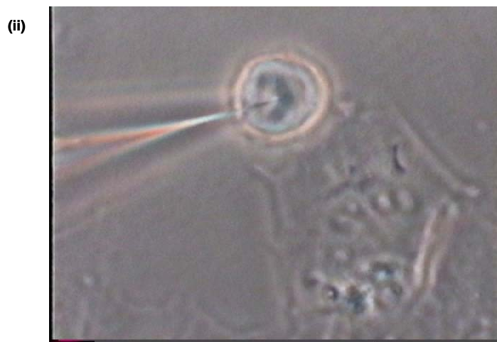
Figure 4.8 shows the intracellular measurement of apoptosis in a single MCF-7 cell. The top image (i) shows an optical nanosensor prior to insertion and a single MCF-7 cell while the BOTTOM image (ii) shows the optical nanosensor inserted into the MCF-7 cell.
