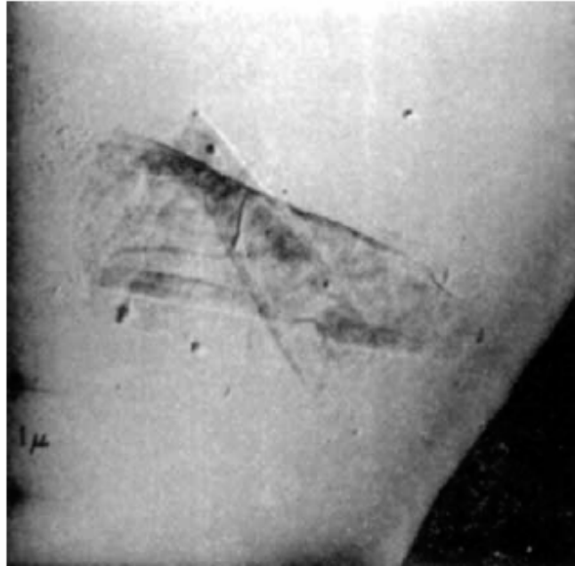
Figure 2.18 Lamellar structure of PA 66 single crystal (Geil 1960).
