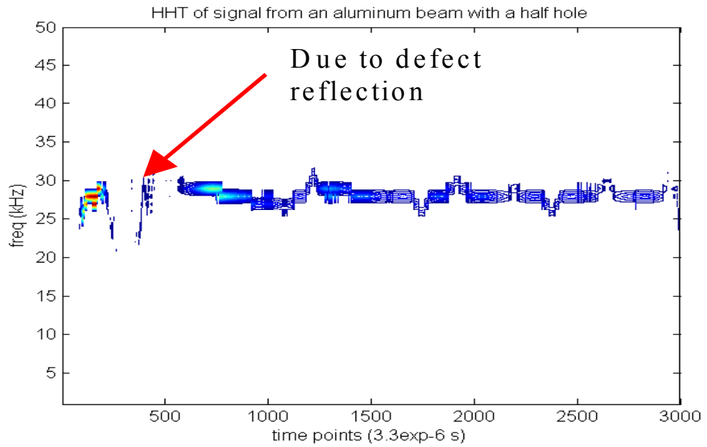
Figure 6.6. Time-frequency representation of HHT of Lamb wave signal in an aluminum plate with a partial hole.
