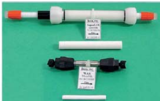
Figure 5. Rod columns (left is polymer columns from Isco, right is silica columns from Merck).
