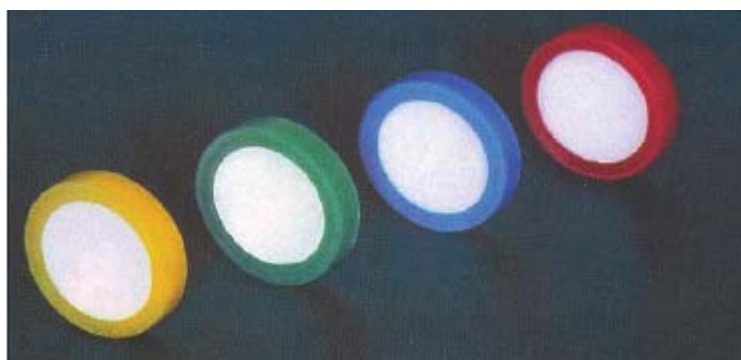
Figure 3. CIM disc columns. The discs are a few mm thick.
