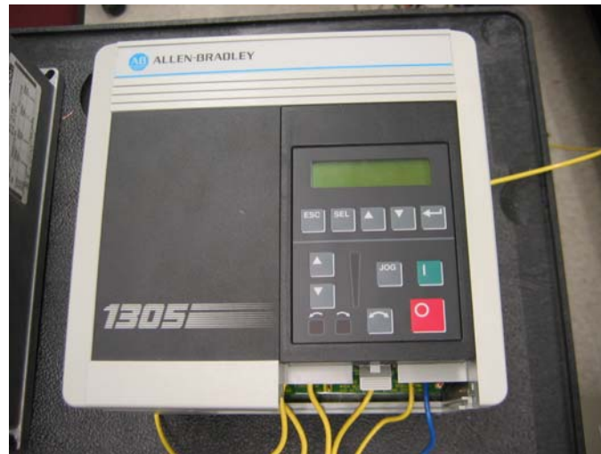
Figure 4.2: Experimental setup of AB1305 inverter.
