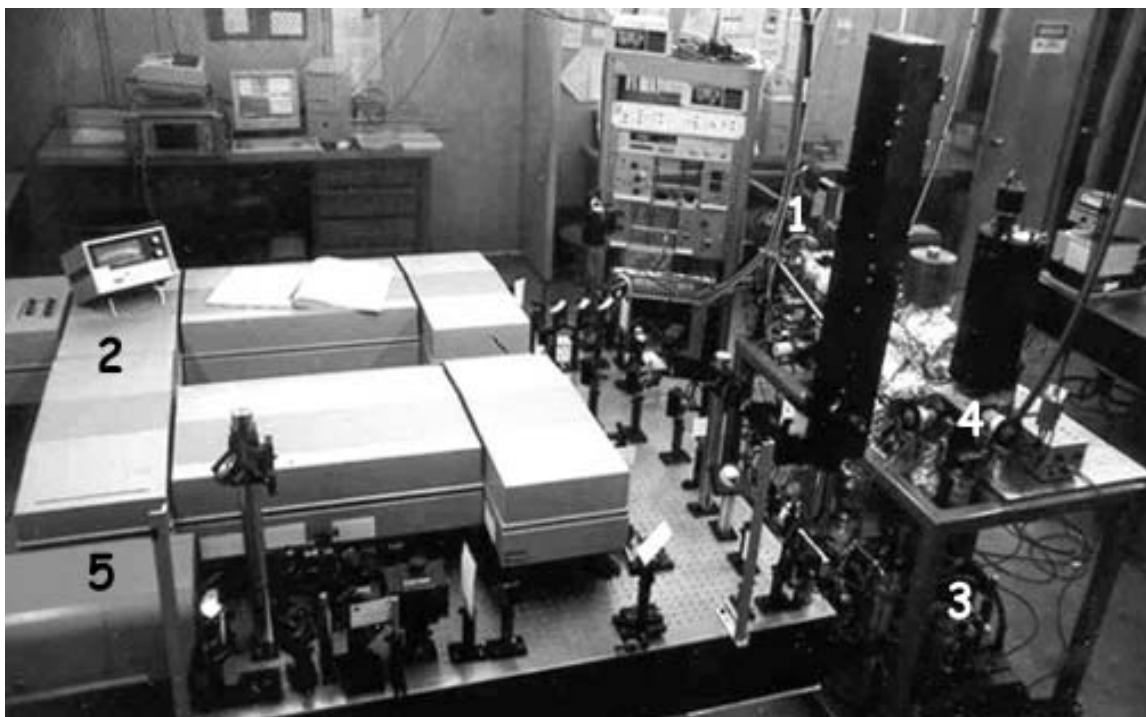
Figure A-1. The laser microprobe resonance ionization spectroscopy time-of-flight mass spectrometer (LM RIS-TOF) as housed at the Institute for Rare Isotope Measurements (IRIM). The numbers (1-5) correspond to the main sections as described in the text.
