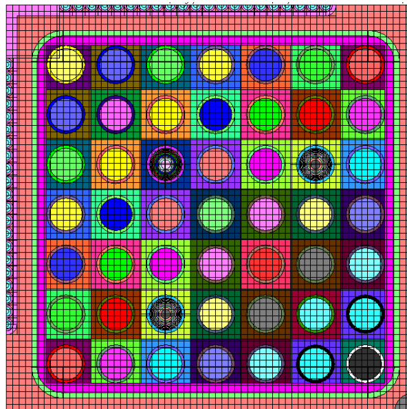
Figure 4.1 – Example BWR lattice generated by TRITON.
