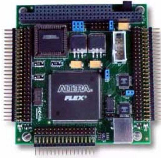
Figure 24. Nova Constellation 10KE Development Board
