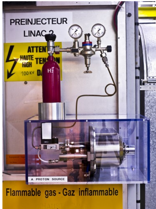
Figure 3.2: The source of protons for the LHC.
