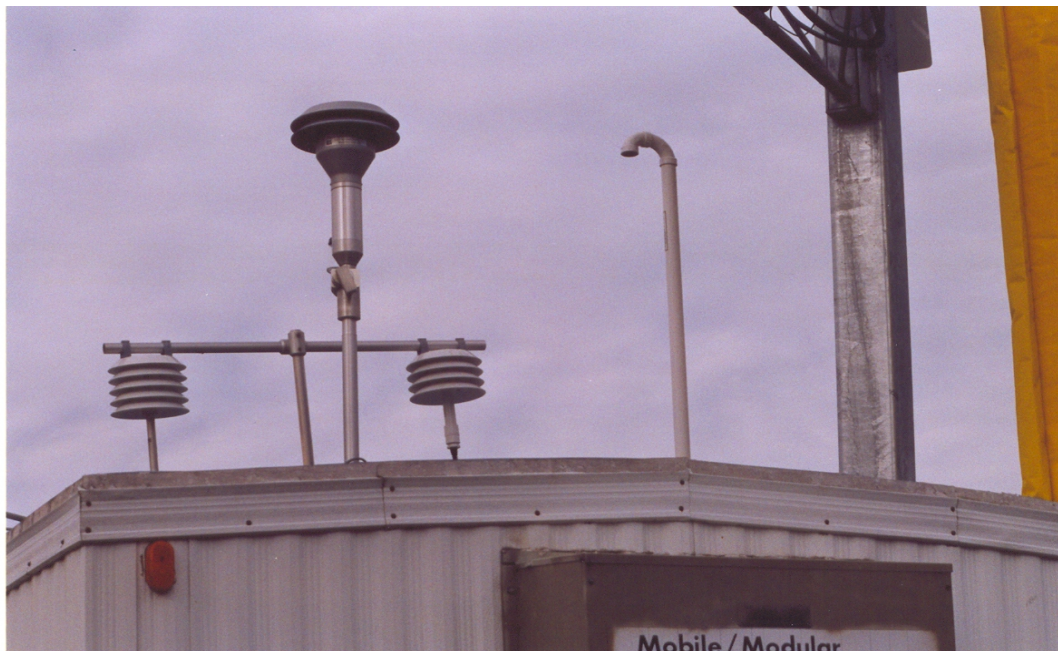
Figure 3.4 Inlets for Sampled Air to the PM 2.5 , NO x and CO Analyzers
