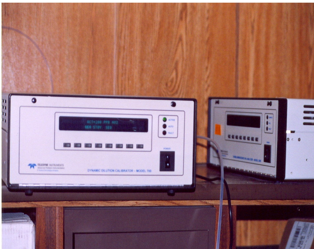
Figure 3.6 NO x Analyzer and Mass Flow Calibrator Inside Monitoring Trailer
