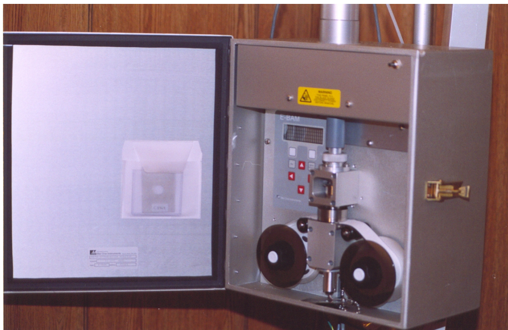
Figure 3.5 E-BAM PM 2.5 Analyzer Inside Monitoring Trailer
