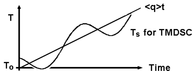
Figure 1.12. A typical heating scan for the sample temperature ( T_s ) of a TMDSC, the line indicated with \langle q \rangle t is linear response. T_0 is initial temperature. Copied from ref. [54].
