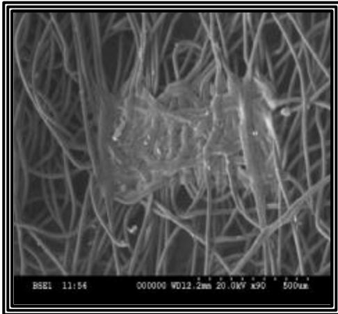
Fig 4.29 SEM Image Showing Re-Orientation of Fibers and Disintegration of Bond at 160° C (Intermediate Stage)
