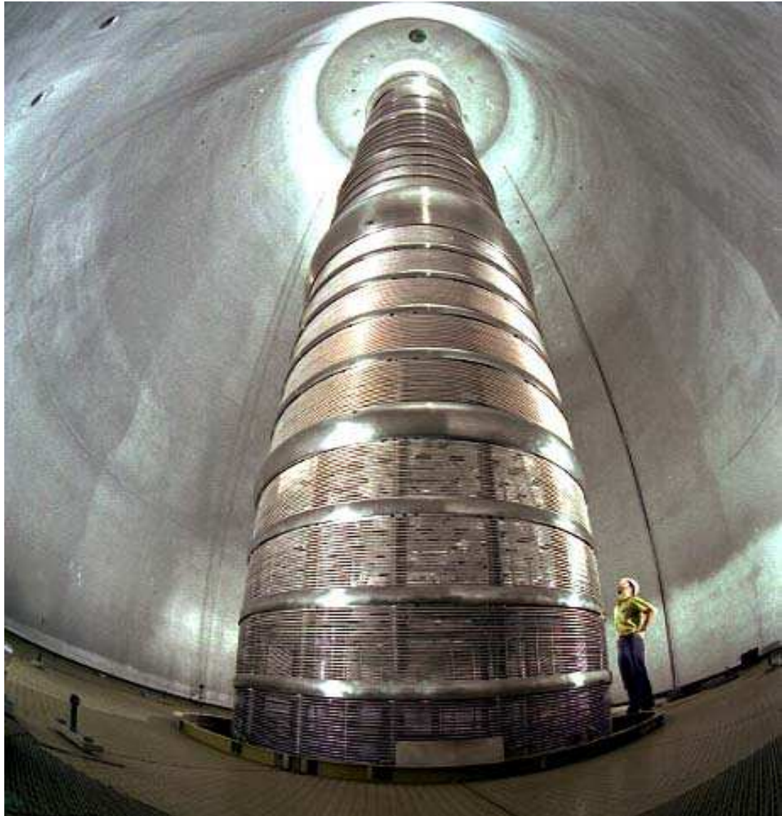
Figure 4.2: A bottom view of the 25 MV tandem electrostatic accelerator.
