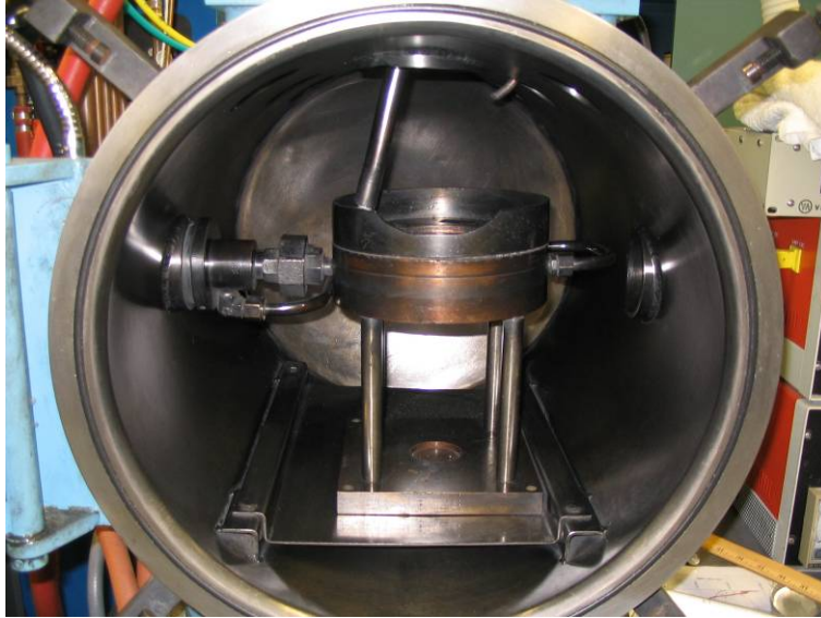
Figure 2.1 The inside of the arc melter chamber. The water cooled jacket in the middle holds the molds. Also seen is the arcing rod.
