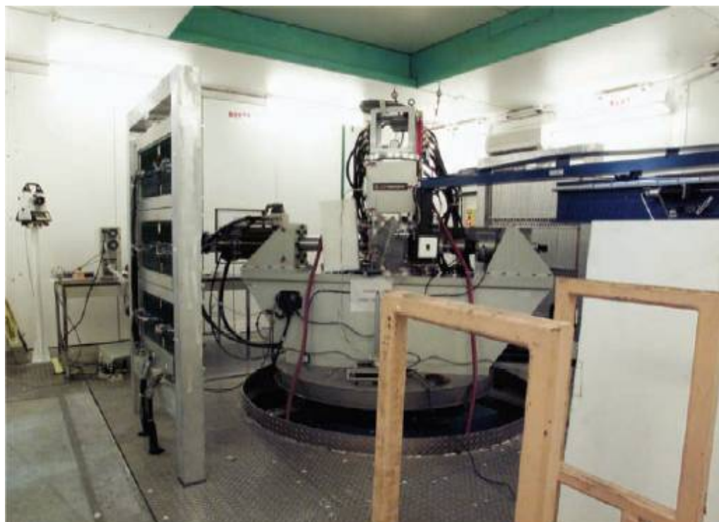
Figure 4.5 Inside view of the SMARTS diffractometer at LANSCE. The load frame can be seen in the centre of the image and the transverse detector bank is on the left.
