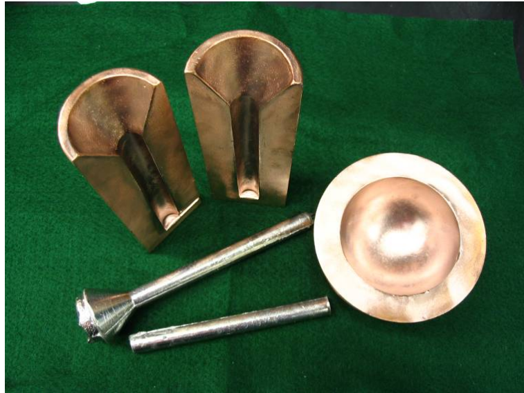
Figure 2.2 Copper molds and cast Fe 3 Al rods.
