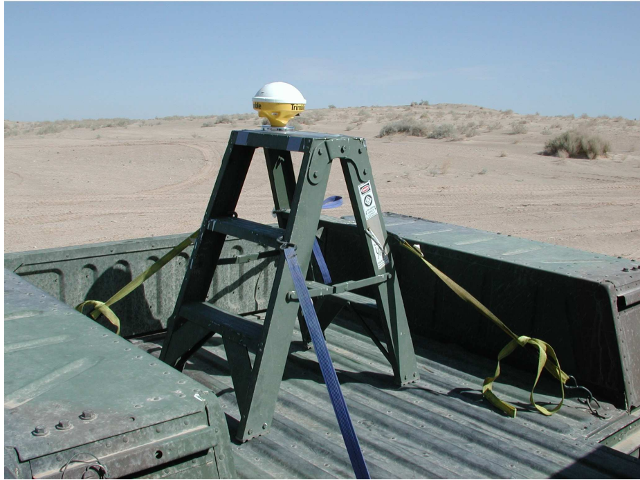
Figure 6.5: Mounting GPS receivers on a HMMWV
