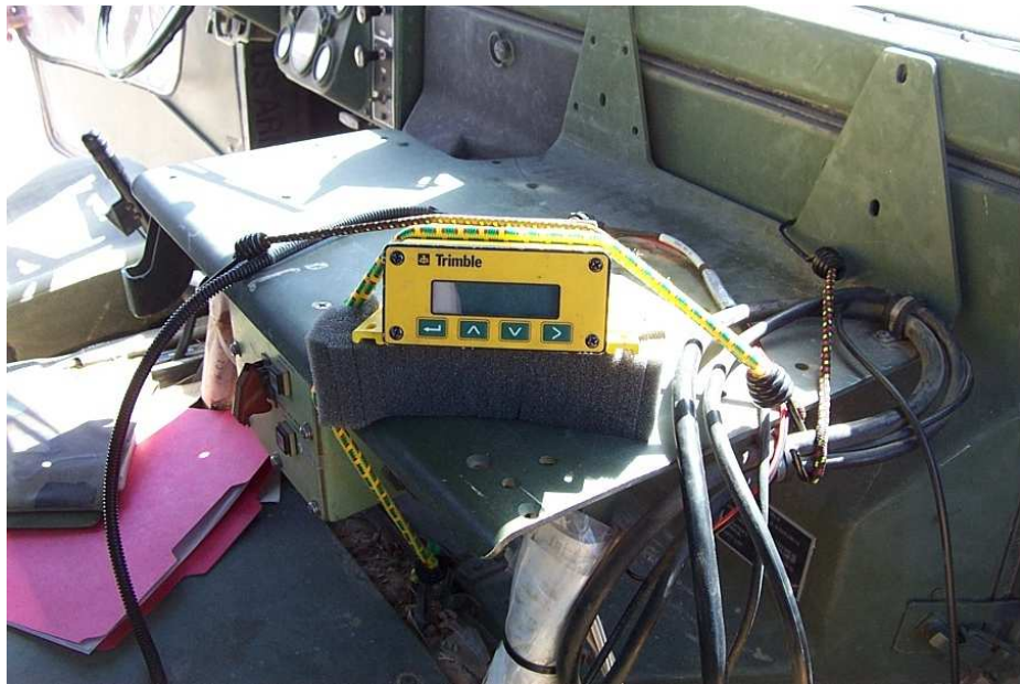
Figure 6.7: Mounting of the control panel
