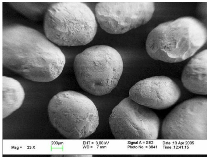
Figure 7.3: SEM image of Ottawa sand particles.
