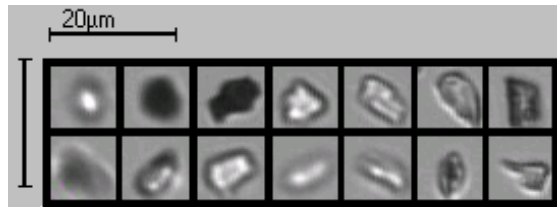
Figure 3.9h: Q-Rok 20 MPa; Size range: 5 - 10 \mu\text{m}
