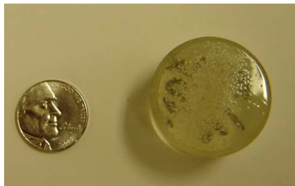
Figure 6.3: Typical sample specimen for nanoindentation on sand particles.
