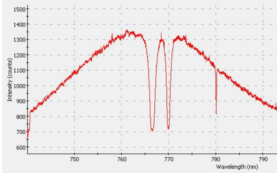
Figure 4.2: D1 (770 nm) and D2 (767 nm) absorption lines of K, and the D2 (780 nm) absorption line of Rb.
