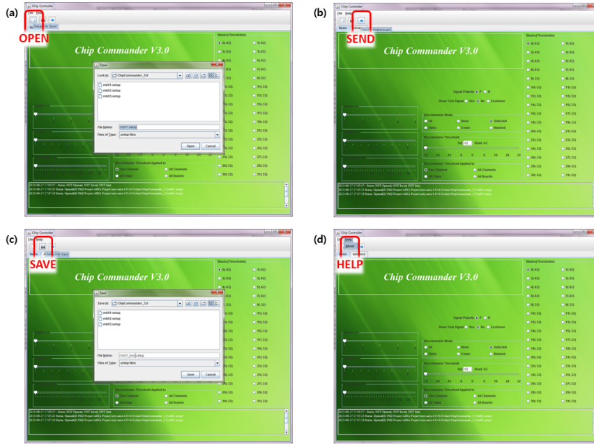
Figure A.12: ChipCommander V3.0 includes functions of open setup file (a), send the file to the XLMXXV and motherboard (b), save the current parameter values (c) and find help on the website (d).
