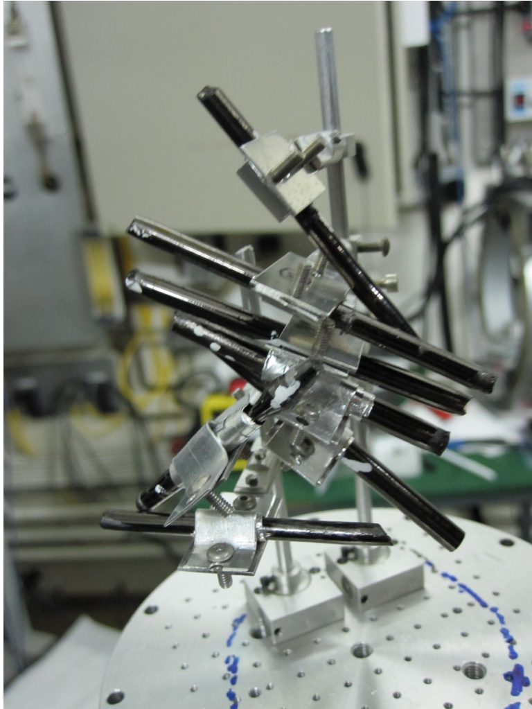
Figure 3.5: An array of aligned PLCCO single crystals, with total mass 25g.
