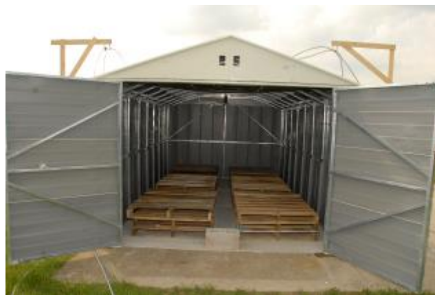
Figure 4.6: Symmetric fuel configuration (PB-1).
