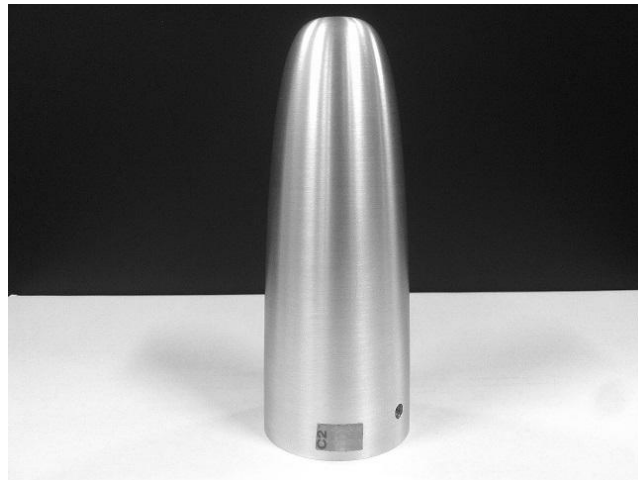
Figure 20. Aluminum BBOR. The biquadratic body of revolution model with r_{avg} = 2.3 \text{ cm} and a length of 12.7 \text{ cm} showing the retroreflective tape and set screw location.
