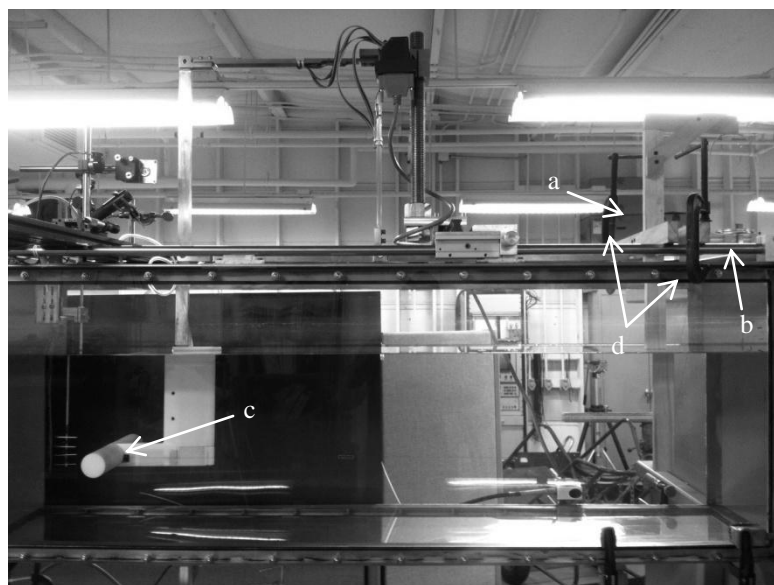
Figure 31. Force Balance Calibration Device Position 2. Shown in the figure are the following: a) force balance calibration device, b) weight basket, c) attachment point to models, and d) clamps attaching force calibration device.
