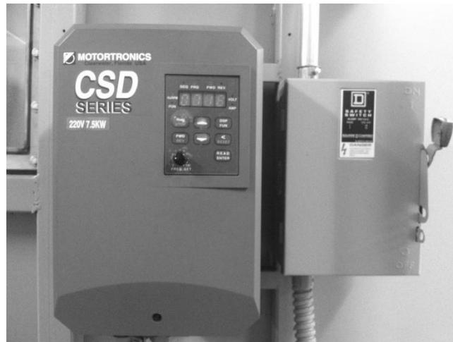
Figure 34. Tunnel Motor Controller. Water tunnel flow speed was initiated and changed by manually adjusting the knob on the bottom left face of the controller.
