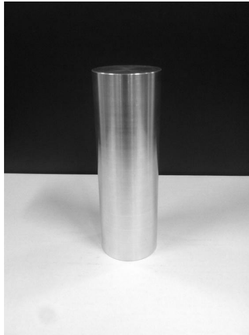
Figure 19. Aluminum CDCC. The constant diameter circular cylinder model with r_{avg} = 2.3 \text{ cm} and a length of 14 \text{ cm} .
