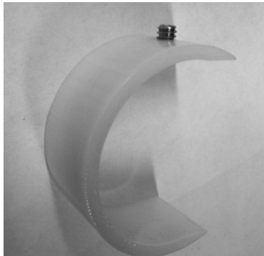
Figure 25. CNF Adapter Cap. The adapter cap with set screw to secure in place when testing BBOR models.
