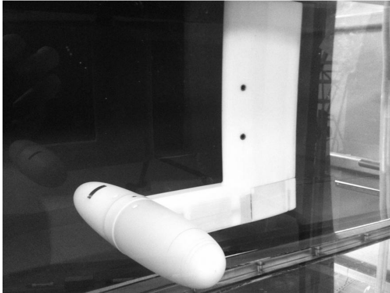
Figure 37. Retroreflective Tape. The BBOR models are installed with the retroreflective tape strip for rpm measurement.
