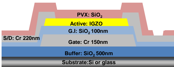
Figure 2-1. The schematic structure of IGZO TFTs (a) Schematic structure of IGZO TFTs with process sequence (b) Layout design of IGZO TFTs (c) Process flow chart of IGZO TFTs
