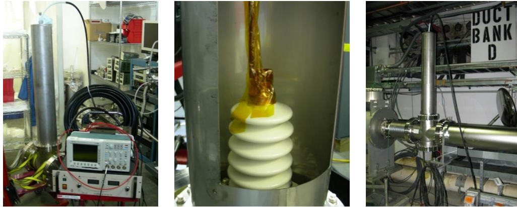
Figure 4.2 (Left) Experimental setup of high voltage test under UHV conditions. (Middle) Air side of the HV bias plate feedthrough with electrically insulating Kapton tape. (Right) Installed IPM test chamber.
