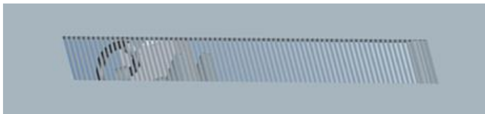
Figure 5.34 Vacuum chamber detector slot with image current path slats.
