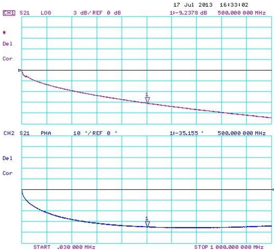
Figure 3.32 Network analyzer measurement of the forward transmission parameter for a 70 m long coaxial transmission line measured from 30 kHz to 1 GHz. (Top) Log magnitude of S_{21} in units of decibels (dB). (Bottom) Phase of S_{21} in units of degrees with 280.13 ns of electrical delay removed.
