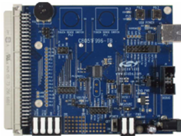
Figure 11. Silicon Labs C8051F996 microcontroller [25]
