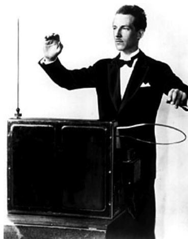
Figure 1. Leon Theremin using mutual capacitance to control volume and pitch.
