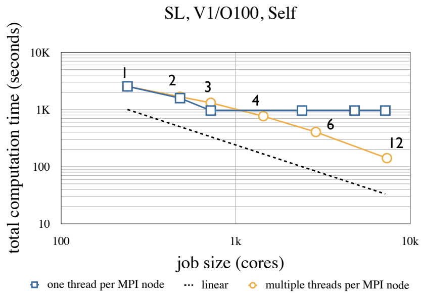
Figure 3.46.: Scalability result using multiple threads for V1/O100 self scattering of the SL system. For clarity the result without using multiple threads is also shown.
