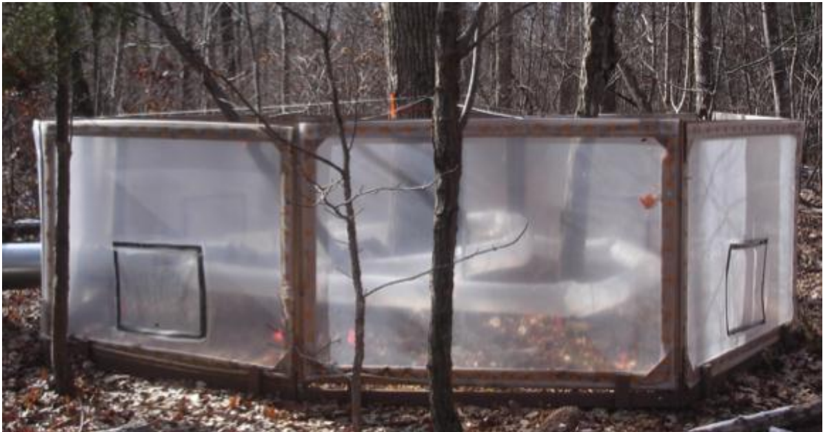
Figure 3. Twelve chambered, experimental plots (chamber volume is 21.7 \text{ m}^3 ) were established in hardwood forests at a southern location and a northern location. A chambered plot at the southern location is pictured above. Plots were warmed using heated air in a regression design at 0.5^\circ \text{ C} half steps from 1.5^\circ \text{ C} to 5.5^\circ \text{ C} above ambient.
