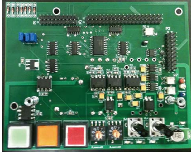
Figure 5.6: DSP interface board circuit revision 1.
