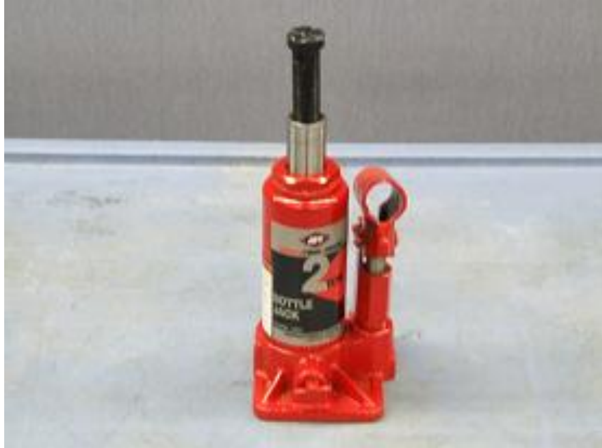
Figure 24. Bottle Jack Used for Water Test Facility.
