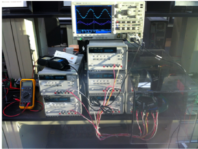
Figure 49 – Eleven-level cascade multilevel inverter setup.
