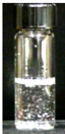
Figure 2-6. Photograph of free thymol suspended at 0.525 %w/v at 20°C after 24 h.
