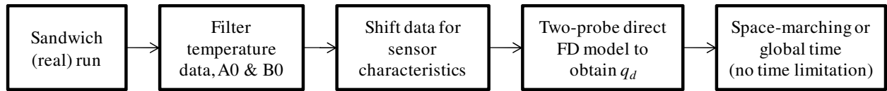
Figure 8.1: Flow chart for preprocessing of data for use in two-probe inverse analysis.
