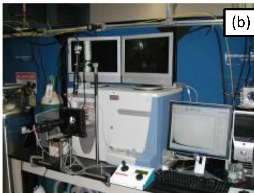
Chp 4 SI 1. Photographs showing the LMJ-SSP setup on LTQ mass spectrometer. (a) Close up view of LMJ-SSP and atmospheric pressure interface region of mass spectrometer. (b) Wide angle view of complete instrumental setup.
